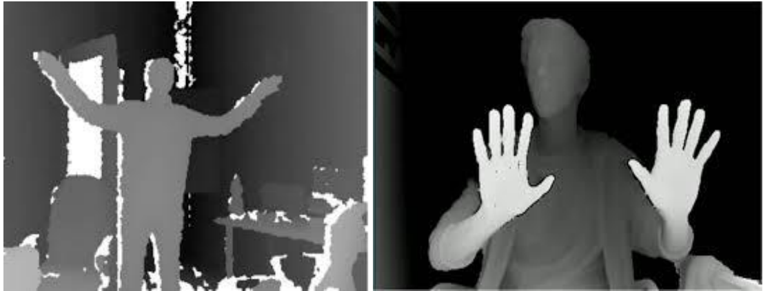
Figure 3.3 KINECT Depth Image
